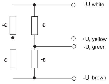
Figure 3: Full-bridge strain gauge
