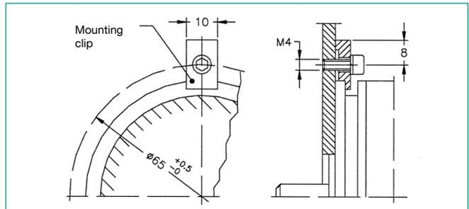
**1 set of mounting angles with screws** (3 are part of delivery) for model 8820-5350 and 8820-5350-V501 **Model 8820-Z002**
